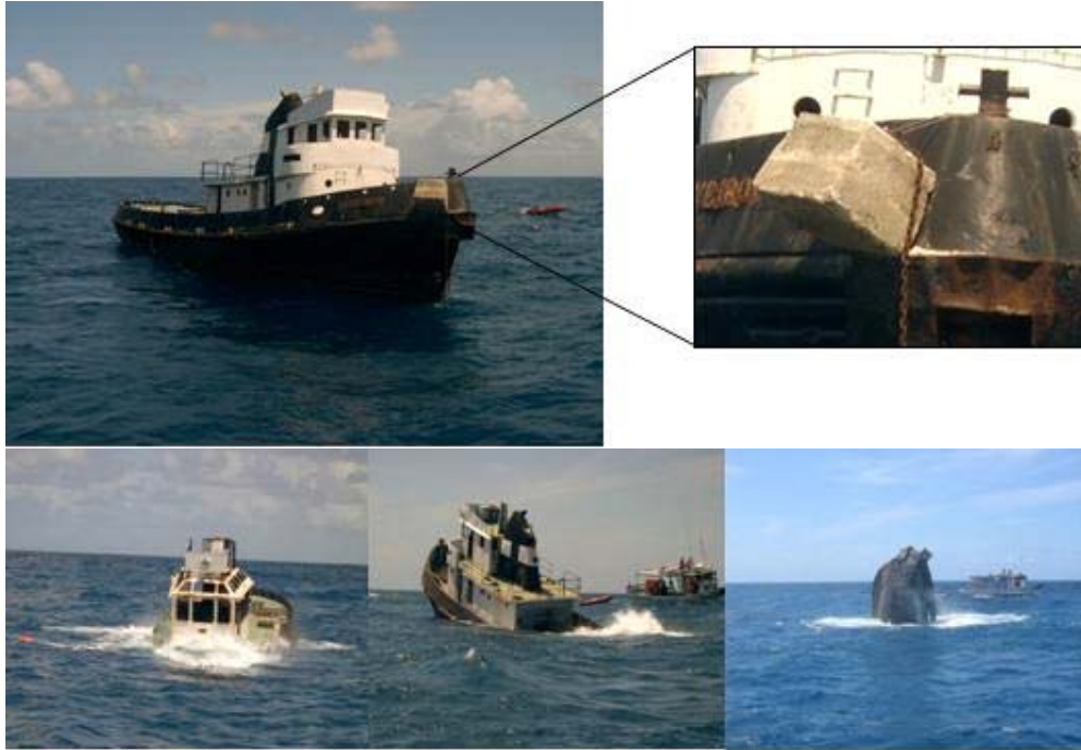
Figure 4 - Detail of the concrete ballast used to anchor the vessels in their sink point.
