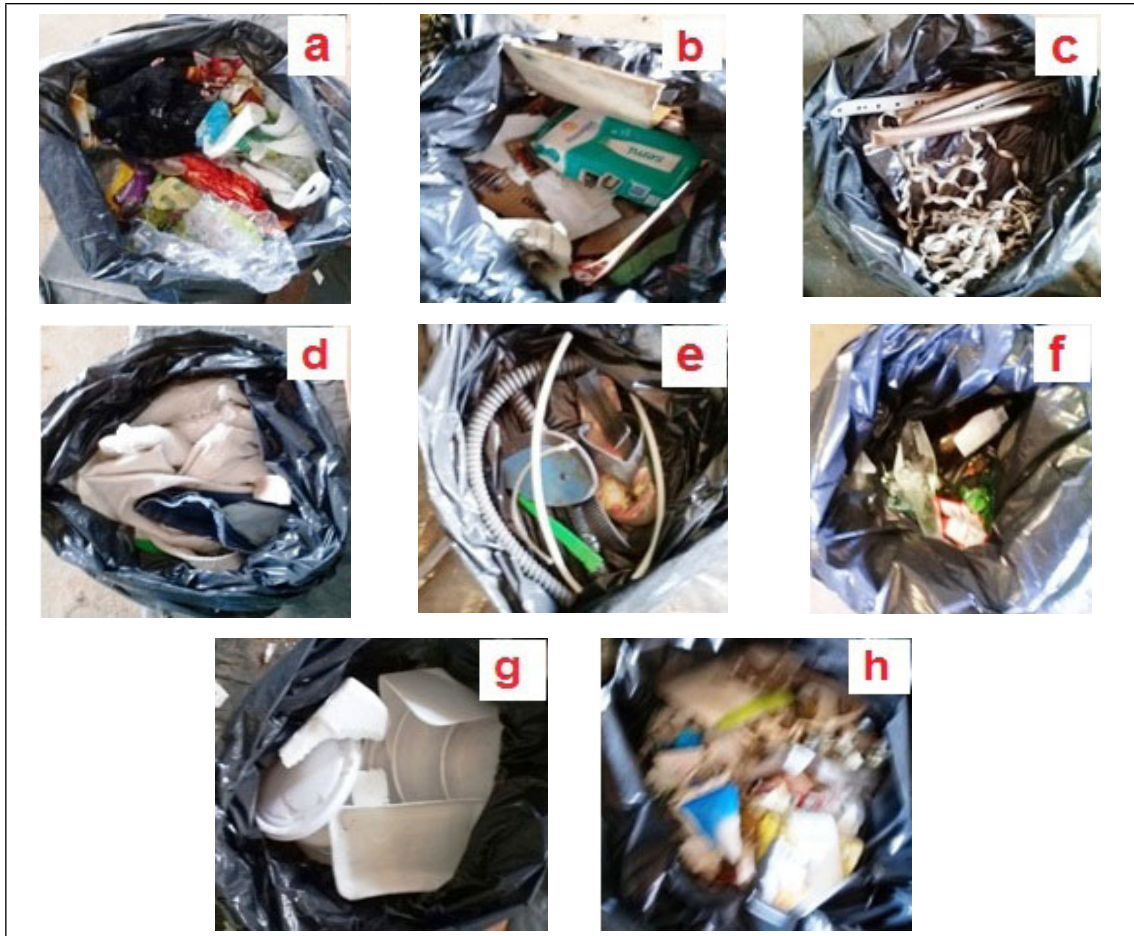
Figure 3. illustrates some of the fractions of dry recyclables and components evaluated in this work. (a) “plastic” fraction, (b) “paper” fraction, (c) “metal” fraction, (d) fabric “fraction”, (e) “rubber” fraction, (f) “glass” fraction, (g) “styrofoam” fraction and (h) “others” fraction.
